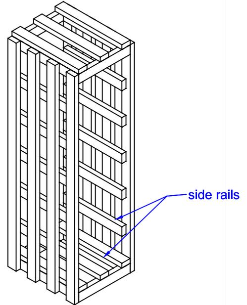
3. Keep adding shelves from the bottom up and nailing them on. Securing the top last.
